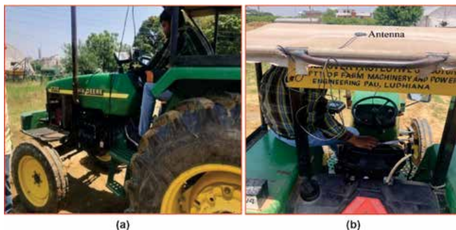
Fig. 3. (a) Installation of satellite navigators ( N_1 & N_2 ) and (b) GPS antenna on tractor
